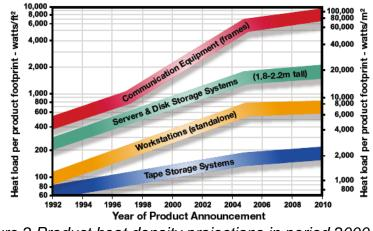
Figure 2 Product heat density projections in period 2000-2010 Source: (Menuet, et.al, 2006, p. 2)
