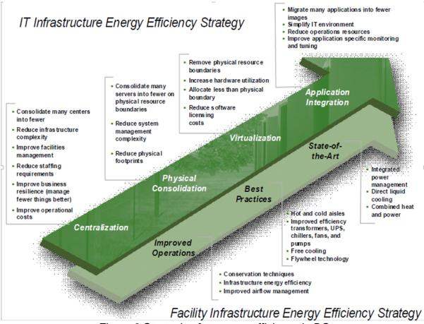
Figure 3 Strategies for energy efficiency in DC http://www.slideshare.net/RahulKaushal/green-data-centerrahul-ppt
